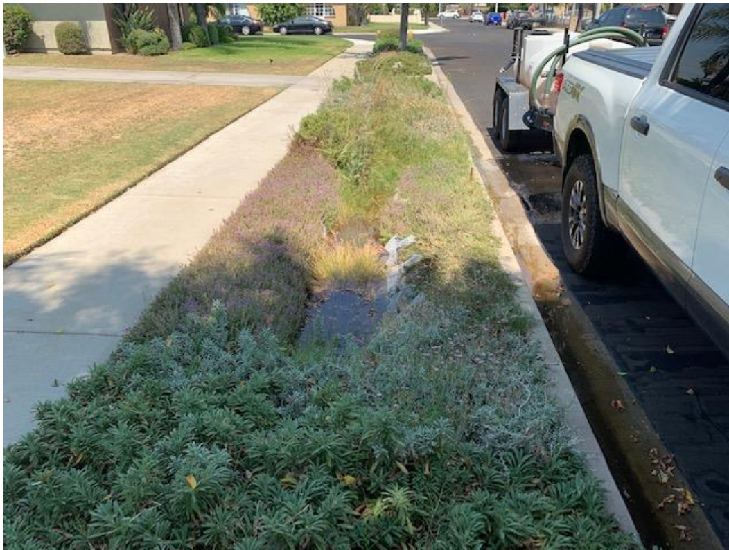
LID Feature during testing
